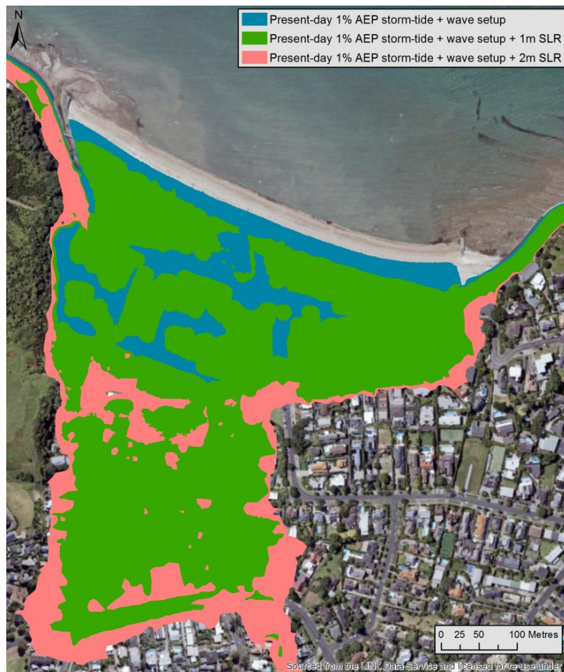
Figure 4. Coastal-storm flood mapping example at Mission Bay, Auckland. Aerial photograph of Mission Bay with present-day 1% AEP storm-tide plus wave setup elevation superimposed (blue shading), plus 1 m SLR (green shading), and plus 2 m SLR (pink shading). After: (50 @Engineers Australia, 2015).
