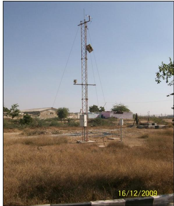
**Figure 6:** Automatic Weather System at Karachi Airport by PMD
