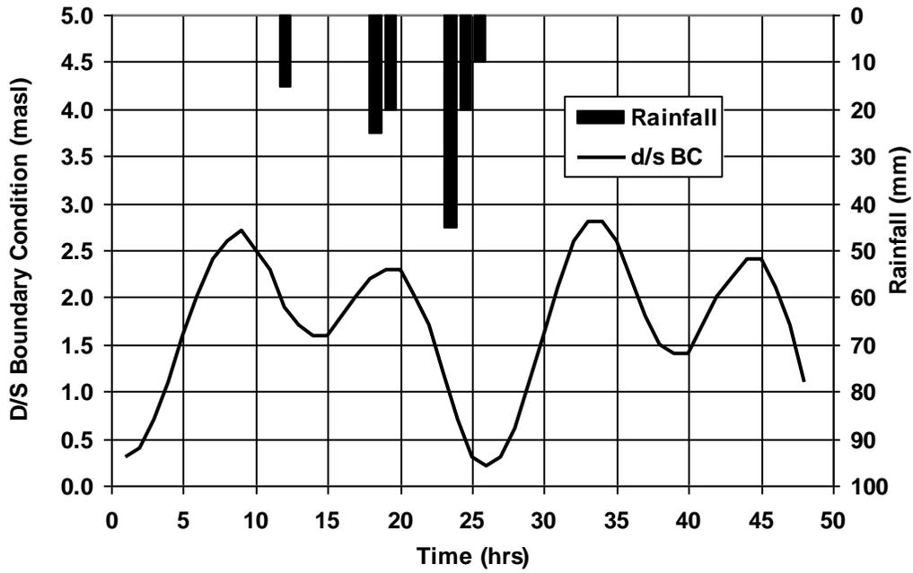
**Figure 11:** Rainfall distribution and oceanic tide levels on 9<sup>th</sup> & 10<sup>th</sup> August, 2007 used for the calibration of the Model
