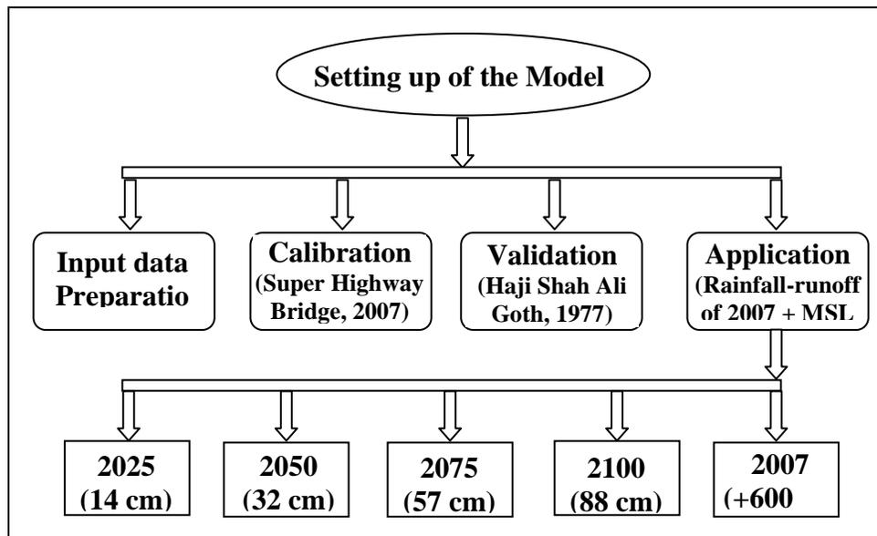
Figure 10: Flow diagram showing the Setting up of the Model for Malir watershed
