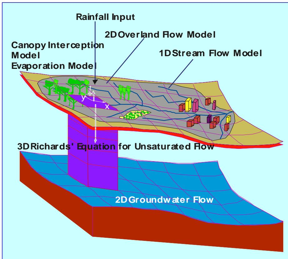
**Figure 2:** Interlinking of various components of IISDHM
