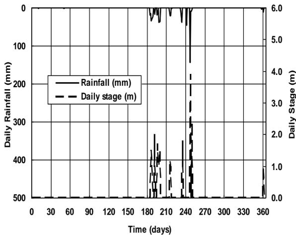
**Figure 5:** Stage hydrograph showing the flashy nature of the floods in Malir River at Super Highway Bridge for the Year 2007
