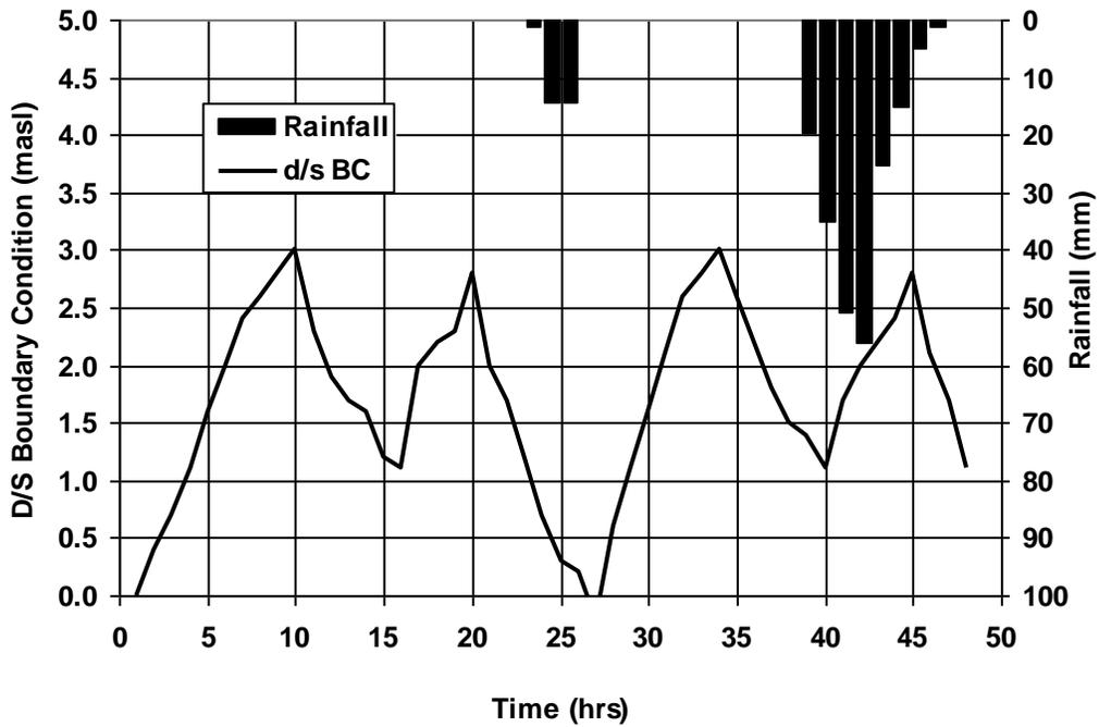
**Figure 12:** Rainfall distribution and oceanic tide levels on 29<sup>th</sup> & 30<sup>th</sup> June, 1977 used for the validation of the Model
