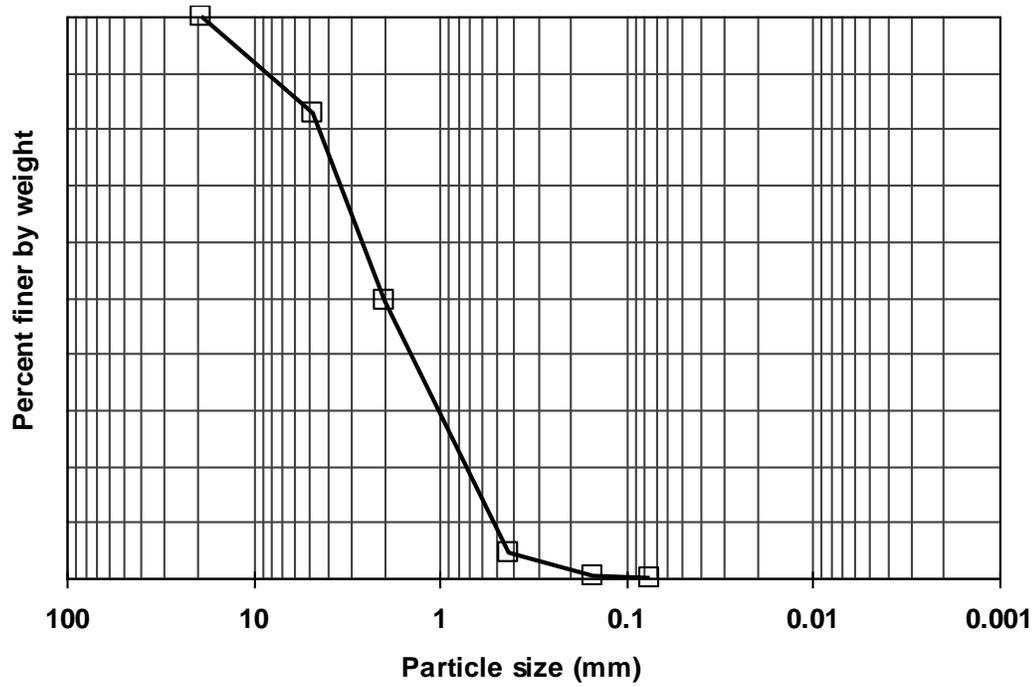
Figure 8: Particle Size Distribution Curve for bed material of river Malir at Super Highway Bridge
