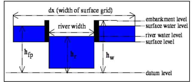
**Figure 3:** Concept of interaction between floodplain and river grid in IISDHM
