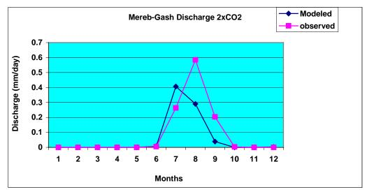
Figure 5.6: Observed and modeled runoff after temperature and precipitation adjustments.
