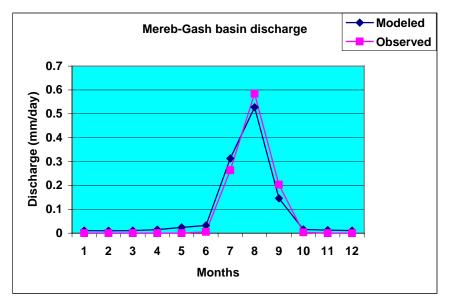
Figure 5.5: Observed and Modeled Discharge Data for Validation of Mereb-Gash Basin
