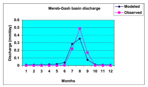
Figure 5.4: Observed and Modeled Discharge Data for Calibration of Mereb-Gash basin
