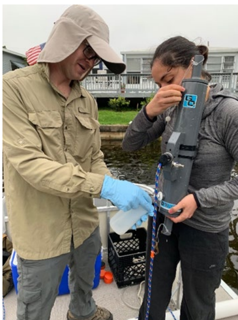
Figure 2-1. Dr. Fox (left) and a student collect water samples in the IRL using a 1.7L horizontal Niskin bottle.
