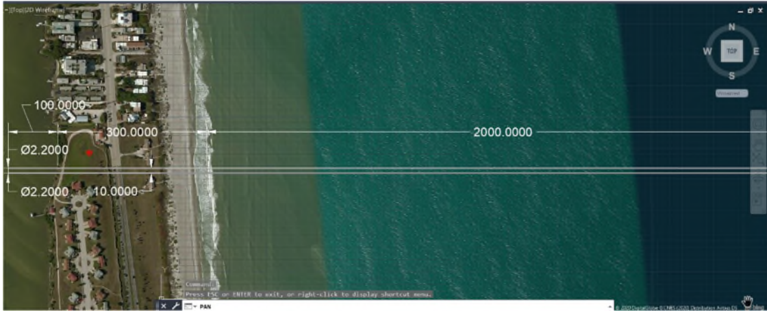
Figure 5-5: Temporary inflow pilot system two pipes no pump (Google Earth 2019)
