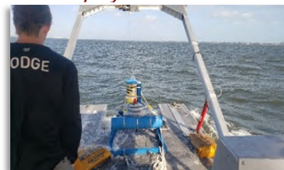
Ekman Grab Sampler (above) and ADCP (below) deployed in the IRL
