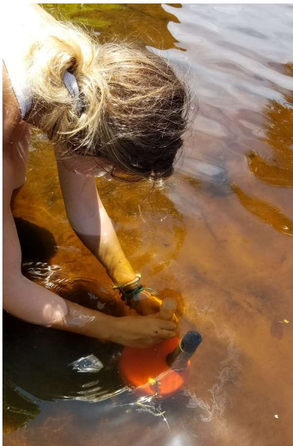
Figure 2-4. Collecting water samples from a benthic chamber deployed in shallow water.
