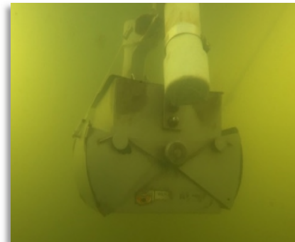
Ekman Grab Sampler (above) and ADCP (below) deployed in the IRL
