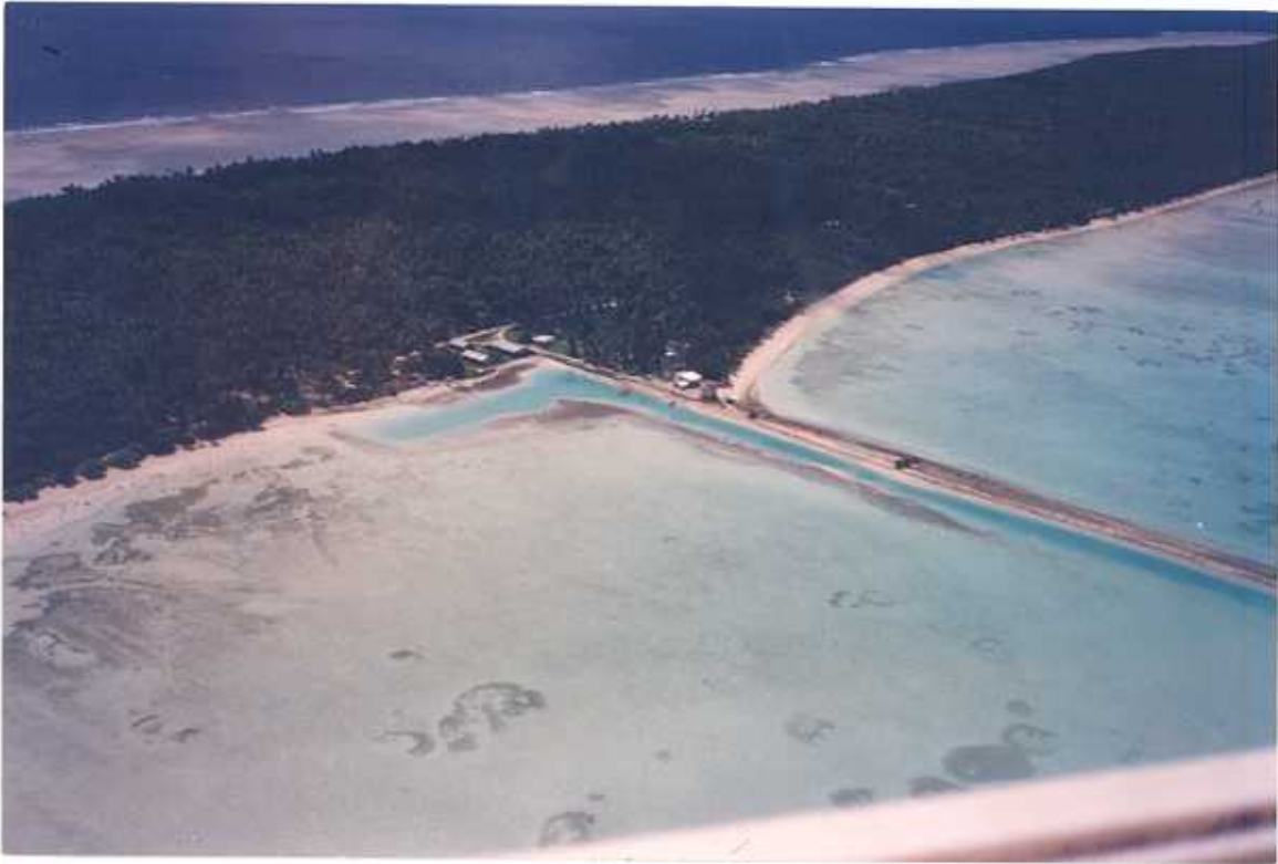
Figure 40. Tanimainiku, Abemama. Oblique aerial view to the southeast showing pronounced shoreline accretion on southeast side of coral rubble mole indicating net longshore transport to the northwest. As a consequence, shoreline erosion has occurred for approximately 300-500 m to the northwest.
