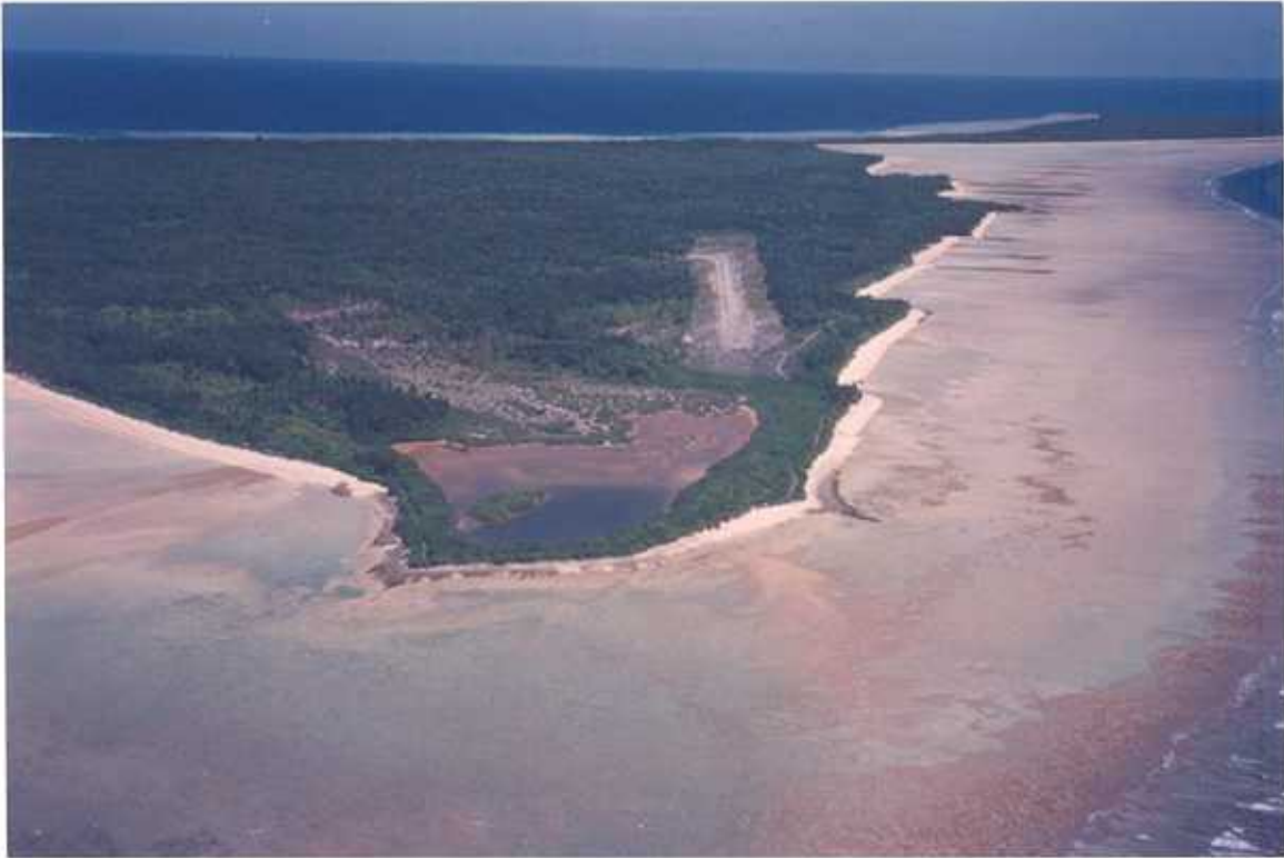
Figure 45. Taubukintekira (east of airfield), Kuria. View northwest along the northeast facing shore of Buariki Island. Area of erosion extends for about 500-600 m along north shore from point of land in the foreground (left centre of photo).
