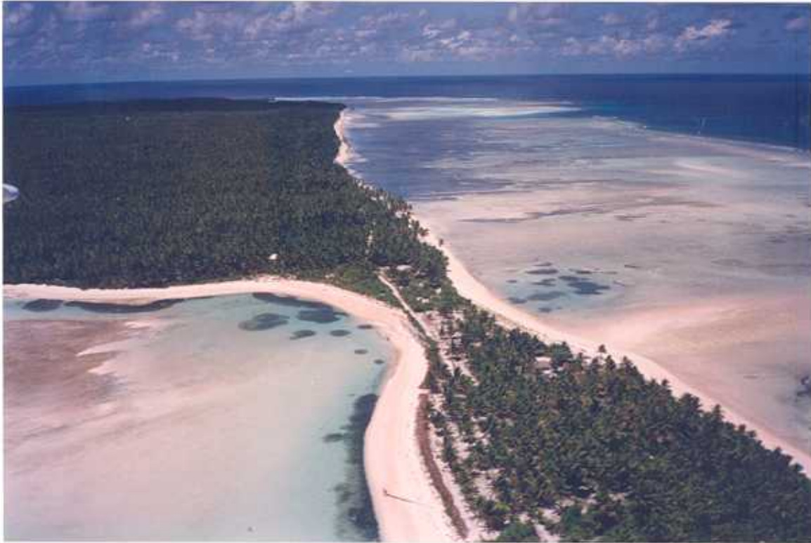
Figure 49. Tanginimake (causeway), Kuria. Oblique aerial view south over site of causeway. Original line of causeway indicated by road on left side. Since causeway completion extensive coastal accretion has occurred on both sides, especially to the west(right) side.
