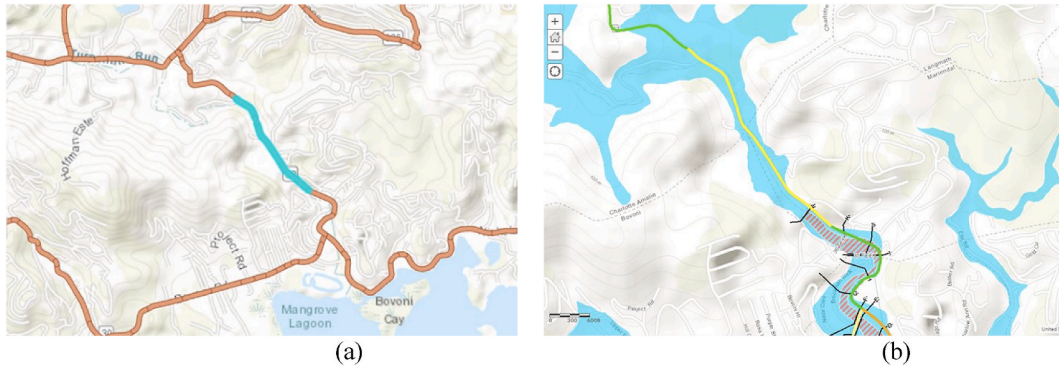
Fig. B8. Segment 2, Route 32 (Turpentine Road) (a) highlighted on road map and (b) overlaid on FEMA NFHL map.
