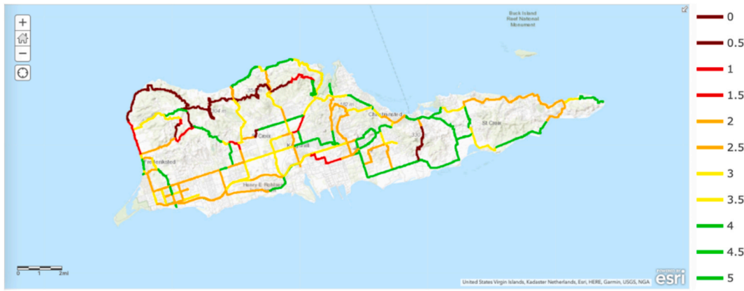
Fig. 5. Colored pavement PSI rating of major roads in St. Croix, USVI.
