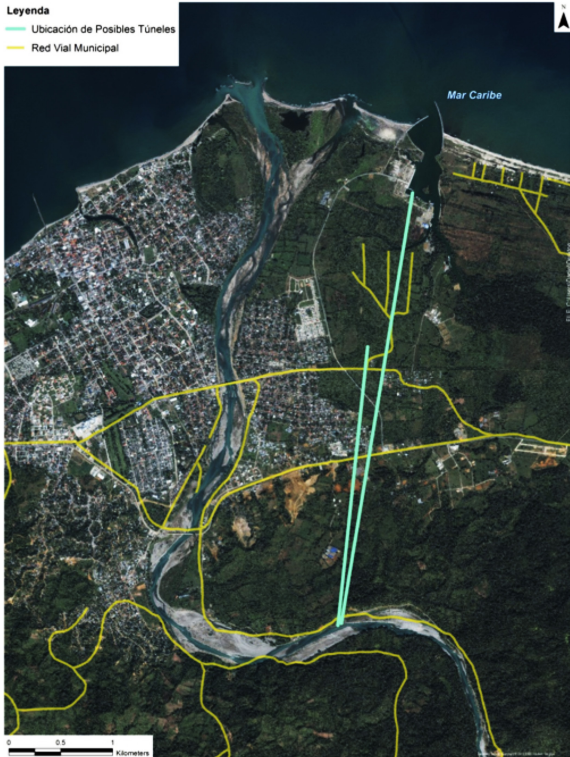
Figure 5-15: Adaptation No. 4: Location of artificial tunnel
