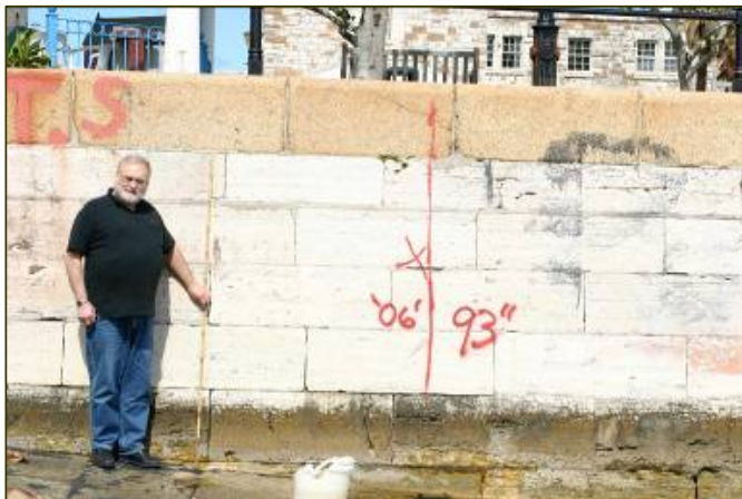
Photograph 3. Steve Blasco measures the Naval Dockyard wall to calculate current sea level from the scum line for comparison with archived photographs from 1876. (Source: P. Rouja).
