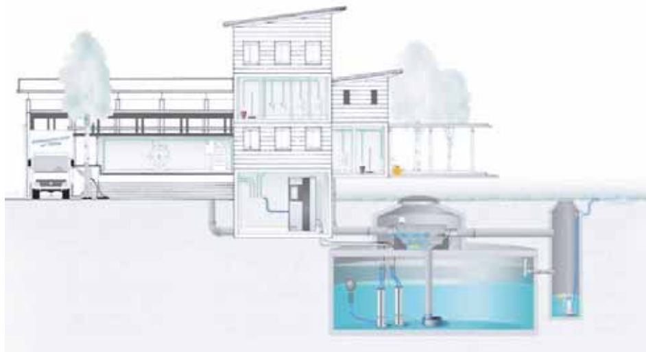
Figure 57: Rainwater harvesting system used at Belgian train maintenance depot (Source: Aquality Trading and Consulting Ltd.)
