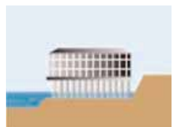
Figure 20: The International Stadium Yokohama was built elevated on pillars so that flood water can flow under it. (Source: Keihin Office of River Kanto Regional Development Bureau 20 ).
