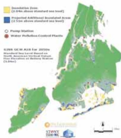
Figure 61: Inundation of New York in December 1992 storm surge compared to a projected inundation in the 2050s taking account of mean sea level rise due to climate change (Source: New York City Department of Environmental Protection).
