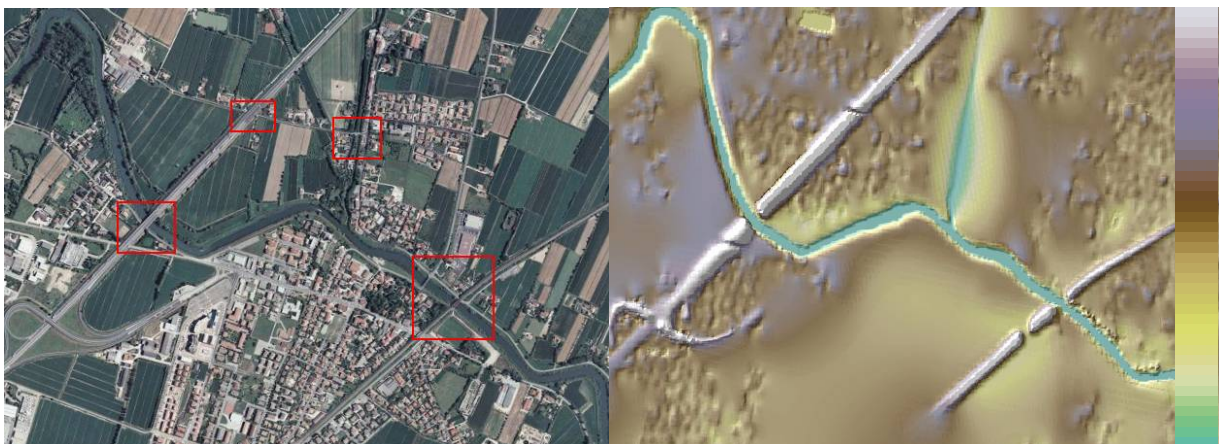
Figure 3: Left: Quarto d'Altino with red boxes to show roads crossing watercourses and other roads (Bing Maps © 2011 Microsoft Corporation and its data suppliers); Right: Quarto d'Altino as represented by the Digital Terrain Model showing the overpasses digitally removed to permit through-flow with colour legend for elevation of the DTM (lilac/light purple shows high elevation, greens show low elevation).
