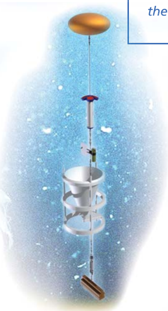
Scheme of a mooring with, from bottom to top: anchor weight, acoustic release mechanism, sediment trap, current velocity meter, acoustic Doppler current profiler and a floater to keep the cable in an upright position. Image: Harry de Porto (NIOZ).
