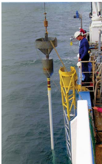
The piston corer is used to collect sediment cores of up to 15 m length. The sea floor is the archive of the oceans, which may be many millions of years old.
