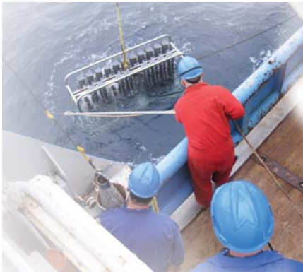
The Titan CTD and water sampler is made of titanium and has been designed and constructed in a close cooperation between the departments of Biological Oceanography and Marine Technology. It is used to study the influence of iron on plankton growth in the open oceans.
