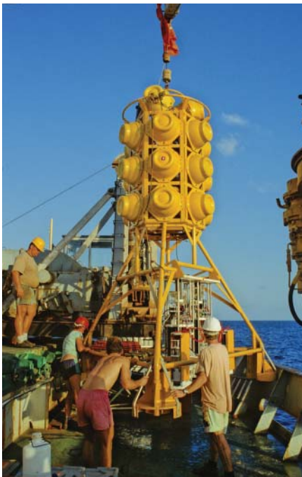
Lander with two ALBEX units to measure the respiratory activity of an enclosed part of the sea bottom. Photo: Gerard Duineveld (NIOZ).
