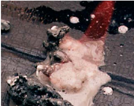
"Burning ice". Gas hydrates are solid ice-like formations with methane and other hydrocarbon inside. When gas hydrate decomposes, it releases methane that can be burned (flame in upper right hand corner). Sample was taken from the Kazakov mud volcano in the Sorokin Trough, NE Black Sea. Courtesy of Prof. M.K. Ivanov, Training through Research programme, Moscow State University, Russia. NIOZ contributor: Alina Stadnitskaia.
