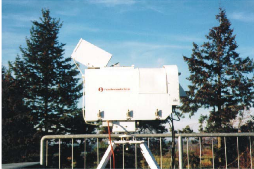
Fig. XI - 2 Radiometrics TP/WVP 3000. Microwave profiler at the MOL-RAO for routine calculations of temperature, humidity and liquid water profiles up to a height of 10 km.
