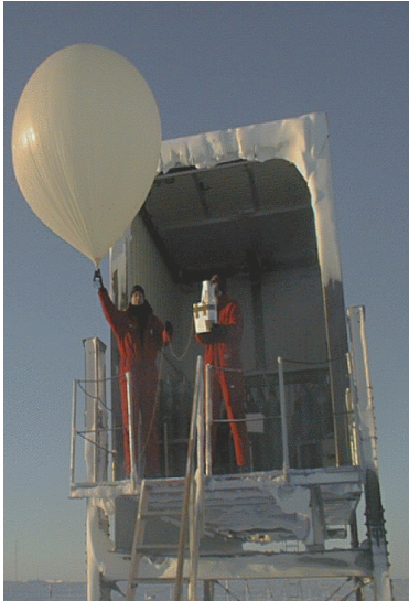
Fig. VIII.6.6.4 Launch of a radio probe at the Neumeyer station
