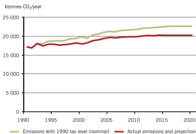
Figure 4.5 Historical emissions of carbon dioxide from the road transport sector and estimated emissions without introduced vehicle fuel taxes since 1990 36 .
