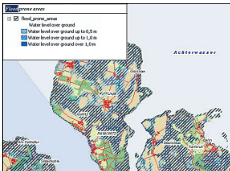
Figure 11: Illustrative map of the peninsula of Usedom showing flood-prone areas at different flood heights (GIS IKZM Oder)
