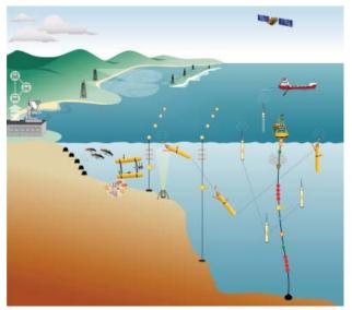
Diagram illustrating how the national IMOS program works. IMOS integrates several independent technologies and instruments, ranging from moored sensors and deep sea autonomous floats, to acoustic tracking devices, radar imagery and remote satellites, among others, into research infrastructure covering a vast swath of Australia's large coastal and deep water marine territory. IMOS will generate critical data needed to support a diverse range of marine research projects.
