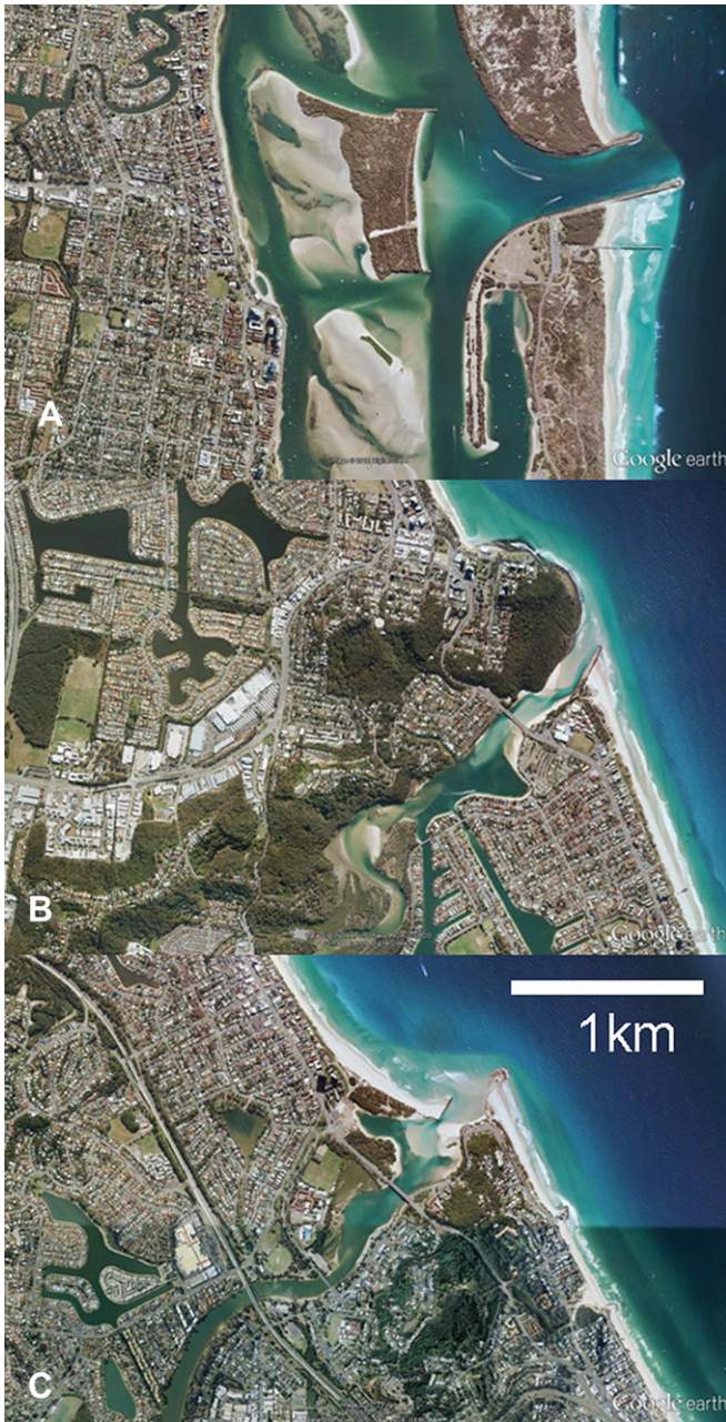
Fig. 4. The tidal inlets of the Gold Coast. A. Gold Coast Seaway, B. Tallebudgera Inlet and C. Currumbin Creek. (Images from Google Earth). All inlets have been stabilized by jetty construction and are routinely dredged.
