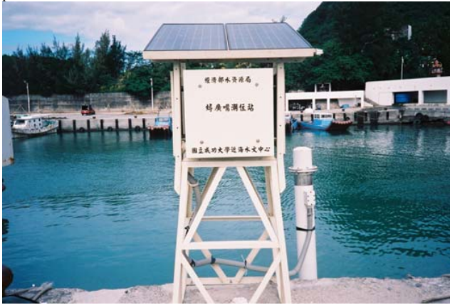
Figure 1 The NOAA-like next generation tide gauge at Taiwanese coast
