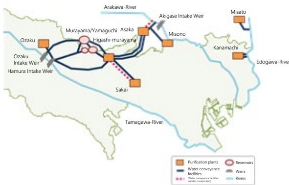
Doubled water conveyance facilities
