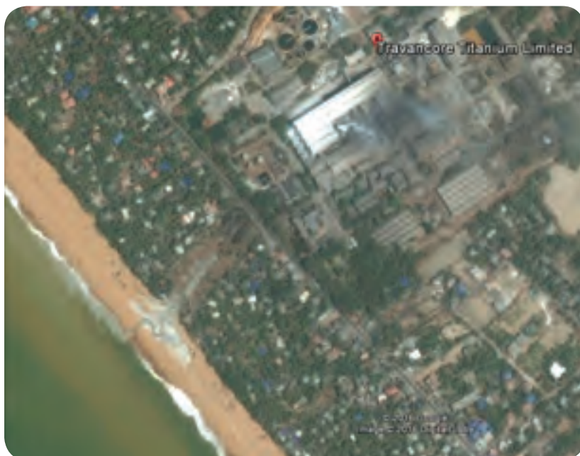
Figure 17. Polluted effluent from Travancore Titanium Products Limited is discharged directly onto the beach at Veli, Thiruvananthapuram instead of further offshore (Guideline F9)
