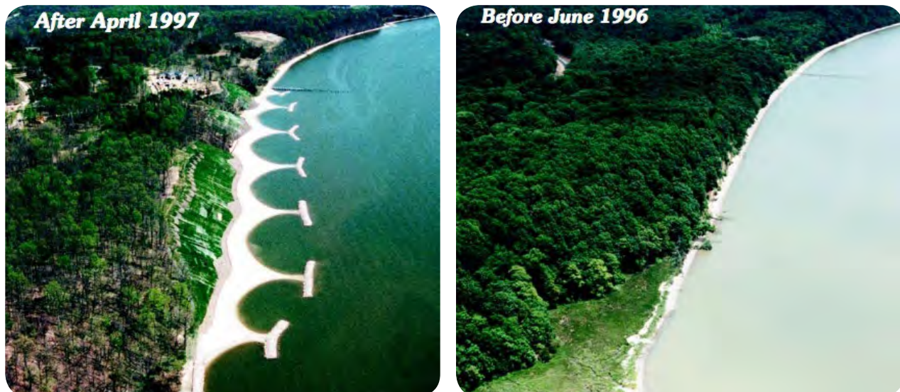
Figure 15. A successful case of offshore breakwaters combined with beach nourishment and beach planting
