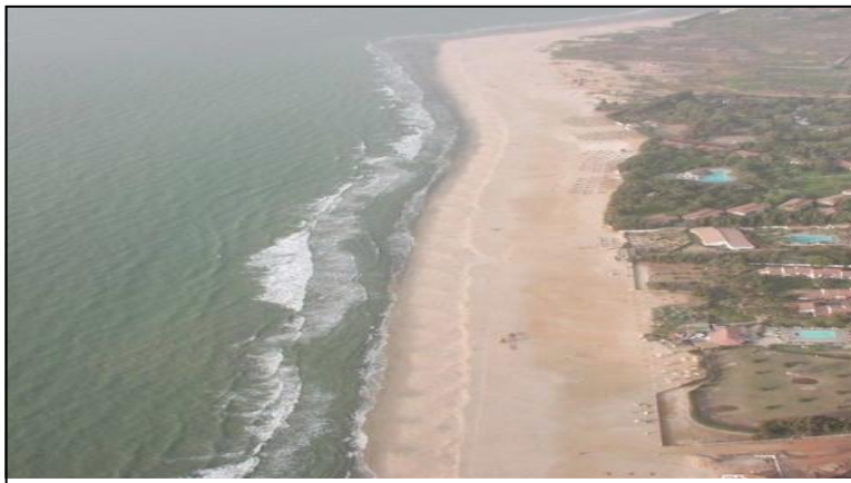
Figure 5.26: Aerial view of Kairaba and Senegambia seafront after completion of beach nourishment project. Beach face is 150 metres wide at high tide. (Photo: Haskoning, 2004).
