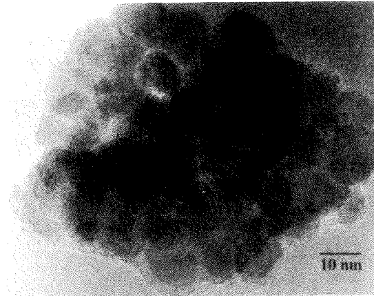
Figure 9. TEM micrograph of region in Co-Mo/tol/H 2 -Ar material containing unusually large particles.
