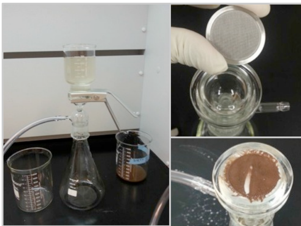
Figure 7: Left: Filtration set up, Right top: Metal screen atop funnel and below storage vessel, Right bottom: Large debris caught by 40 \mu\text{m} filter on metal screen
