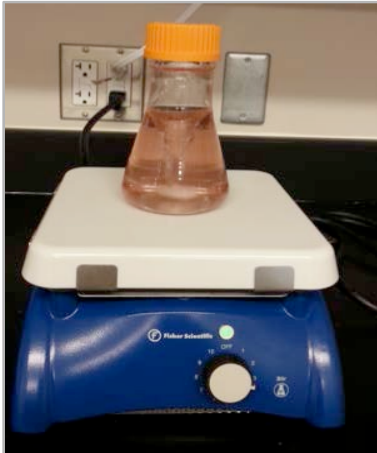
Figure 2: Microspheres stirring with magnetic rod on stir plate
