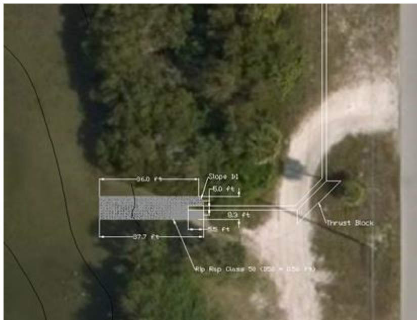
Figure 40. AutoCAD drawing of outflow structure top view
