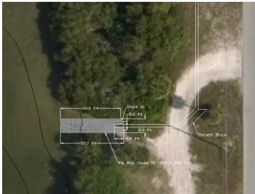
Figure 8. AutoCAD drawing of outflow structure top view
