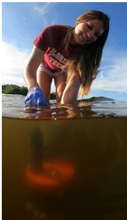
Figure 52. Collecting water samples from a benthic chamber deployed in shallow water
