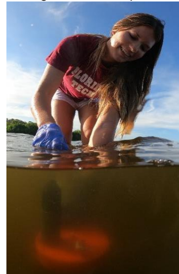
Figure ES-3. Collecting water samples from a benthic chamber
