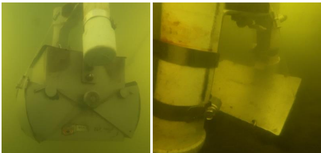
Figure 51. Ekman Grab photographed by scientist with SCUBA descending through the water column (left) and settled in sediments with no visible disturbance to the sample (right)
