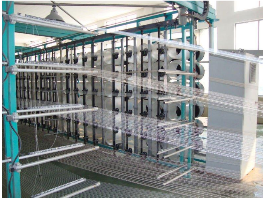
Figure 7.2: Example Creel System [191]
