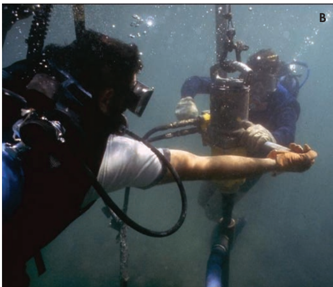
FIGURE 1. Collecting cores from Galeta Reef, Panama, above (A) and below (B) the sea surface with a hydraulically operated drill (photos courtesy of Ian G. Macintyre).
