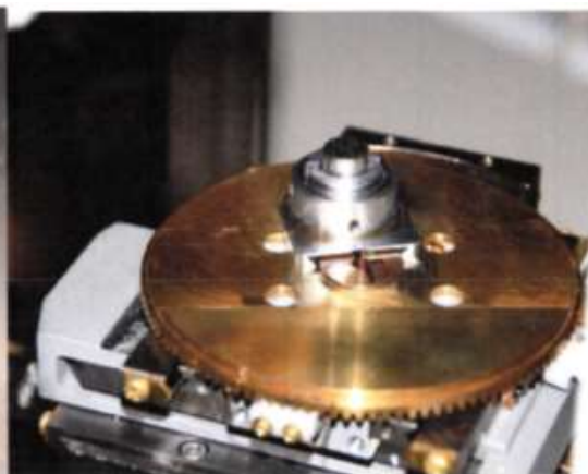
Stage turned for image to show how dovetail fits onto the stage.
